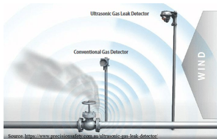
Fig. 10. Functioning of an ultrasonic gas detector
